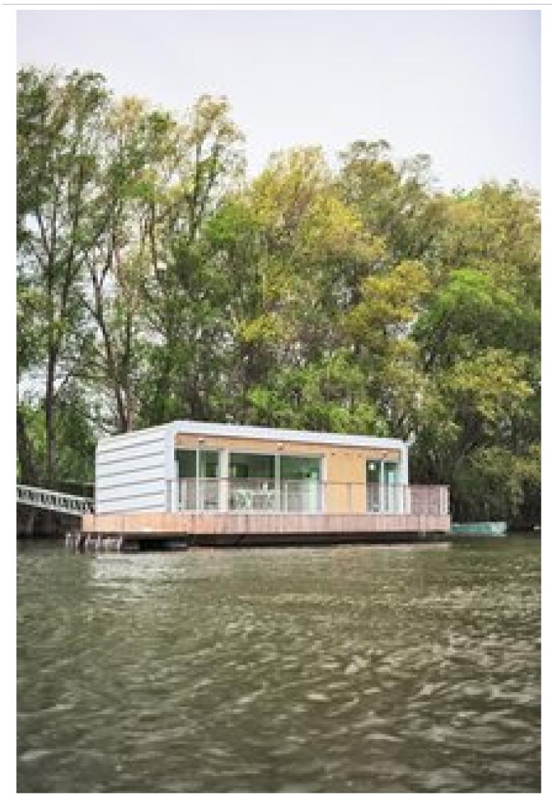
SM Ponton is a Slovakia-based designer and producer of modular, floating pontoon bases for houseboats and floating homes. Constructed with a reinforced-concrete structure that ensures maintenance-free durability and a Styrofoam core that makes the vessels unsinkable, the modules are connected together to form a rigid pontoon platform using locks at the mooring place. Architects and designers can then confidently build their homes on top of this platform.
