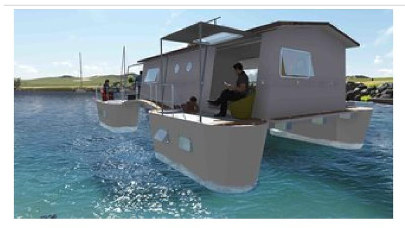
French company Farea manufactures floating homes that are certified as boats. This is important in France, as it means the houses are allowed in lakes, lagoons, and at sea. They're about 915 square feet each and come with five twin cabins, three terraces, and a kitchen. The structures can produce their own water and electricity and are packaged in a 40-foot-long transportable container for international shipments.
